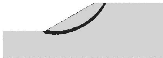
图 1 用塑性应变剪切带表示的滑动面 Fig.1 The failure surface using continuous contours of equivalent plastic strain
